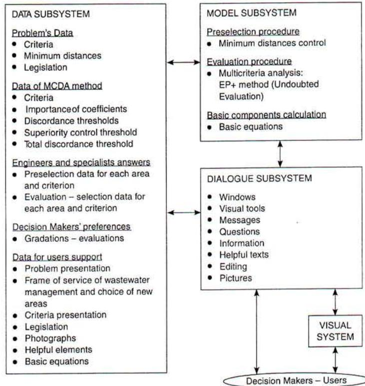
Fig. 2. The components of the suggested tool.
